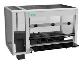
Our Proteograph automation instrument has been configured to process one full 96-well plate at a time. For our first Proteograph assay this translates into processing 16 samples in parallel for each 96-well plate run. Our Proteograph Instrument Control Software (PICS) for the Proteograph is fixed and tailored to our specified workflow. Each new Proteograph assay will be able to run on our same Proteograph automation instrument with a new NP
